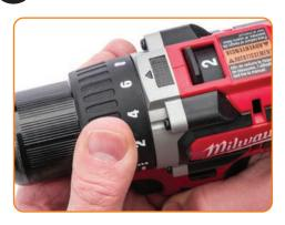
If your drill has a drill and clutch mode, set it to clutch mode. Turn down torque to the lowest setting. Increase as necessary to fully drive screw.
