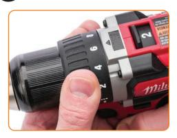
If your drill has a drill and clutch mode, set it to clutch mode. Turn down torque to the lowest setting. Increase as necessary.
